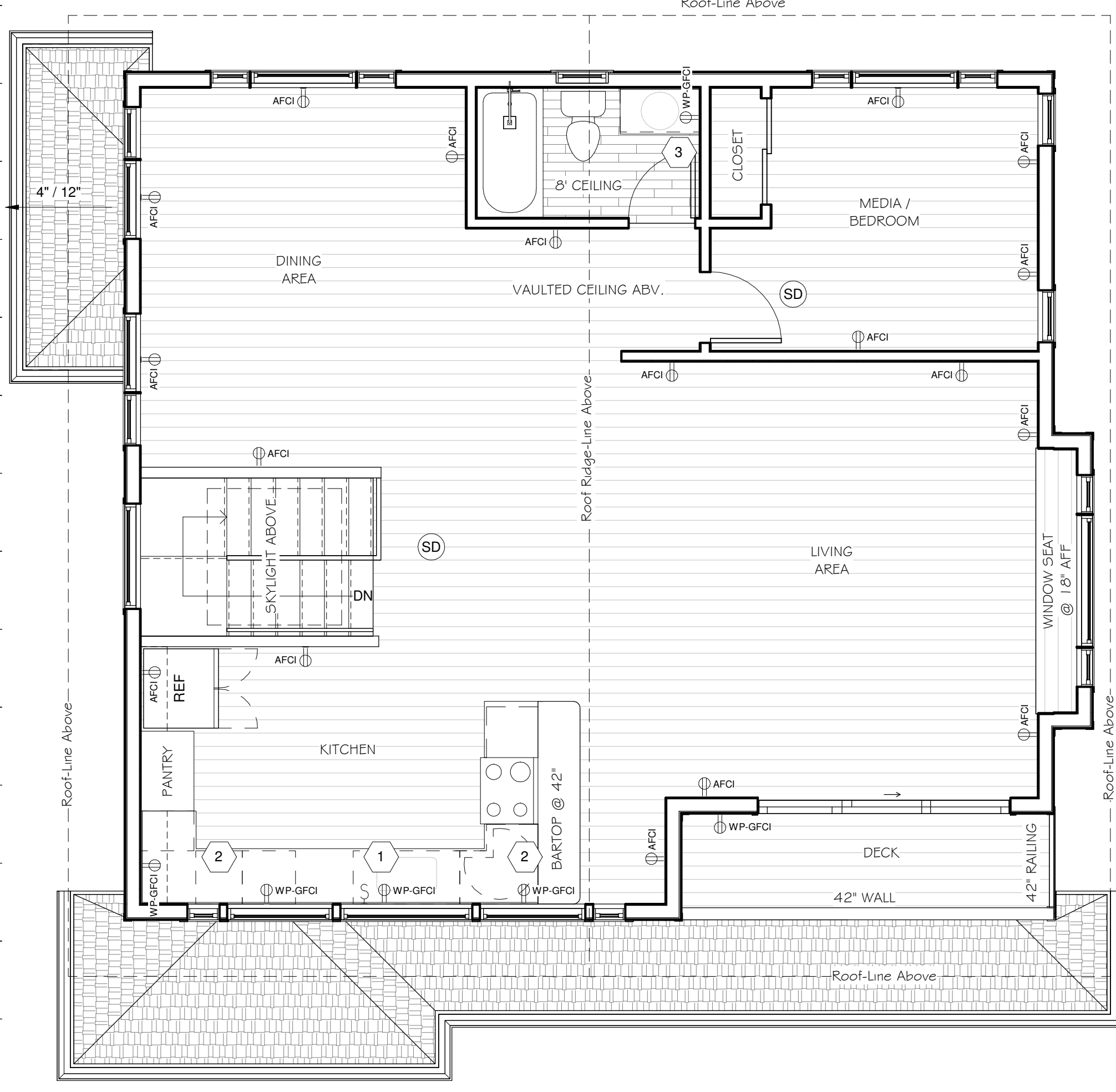
2 Level 2 - Second Floor Electrical 1/4" = 1'-0"
