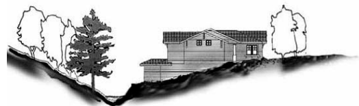
Structure is too close to natural drainage feature
