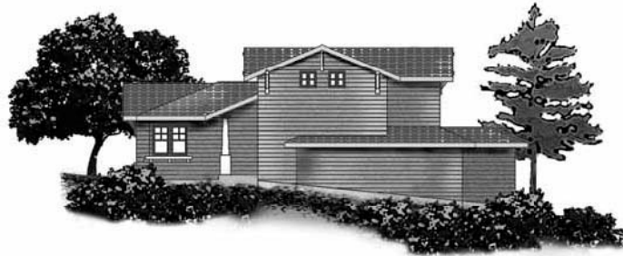
Structure is designed to blend with the natural contours and features of the site. Only grading necessary for construction was used.
